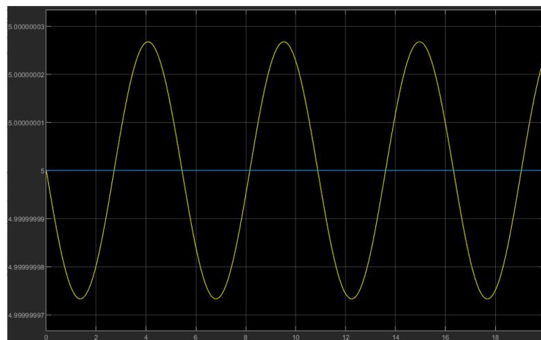
Fig. 4 Robot length graph (blue color is the actual value of the wheelbase of the mobile robot, yellow color is the calculated value)
