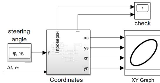
Fig. 2 Simulation diagram in the Simulink environment
