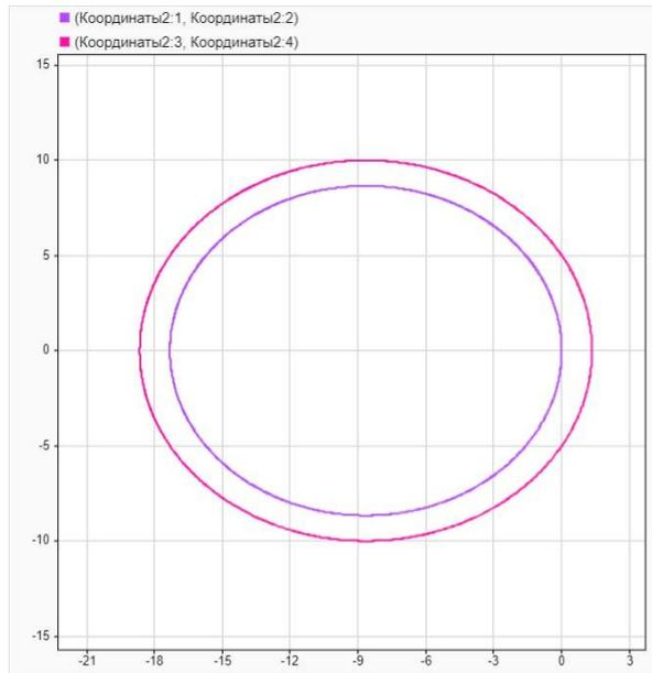
Fig. 3 Graph of the movement of the front and rear wheels (pink color – graph of the front wheel, purple – graph of the rear wheel)
