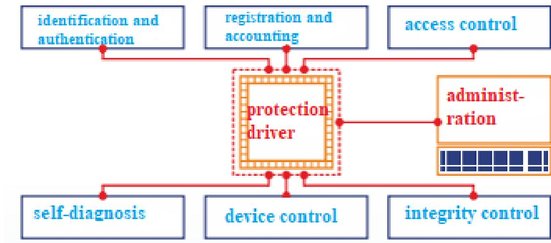
Figure 3 - Functions of the trusted boot tool
